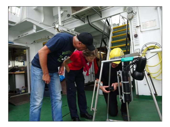
**Fig. 2**. The Eagle has landed – or at least will be landing soon. **Janne Bruun** and **Tarja Katajisto** observing closely the technical wizardry of **Harri Kankaanpää** who is preparing the home-made prototype benthic lander for first testings. This simple but genious gear takes us right to the bottom to visually observe and measure with various sensors what happens down in the depths.
